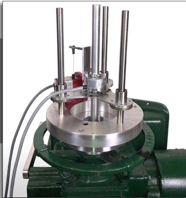
*\*SAMD shown mounted on SMB-000 Limitorque actuator*
